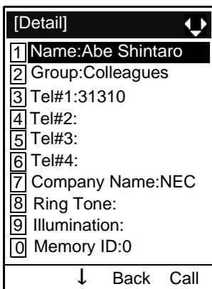
STEP 2: Select a target telephone number and then press (**Enter**), (**Right-cursor**) or **OK** soft key. (or press the appropriate digit key.)
