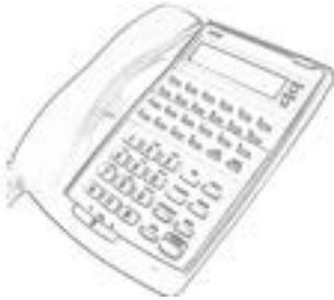
The XN120 system phones can be connected to any of the eight RJ11 telephone sockets labelled ST1 to ST8 in the XN120 unit.
