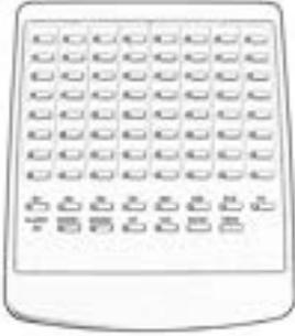
The 64 Button Consoles can be connected to the RJ11 telephone socket labelled ST8 on the XN120 (refer to Appendix A for further connection options). The console must be used in conjunction with an XN120 System Telephone (a display phone is recommended).
