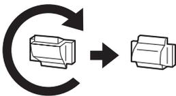
3. Slide the handset hook back into the slot until it locks.
