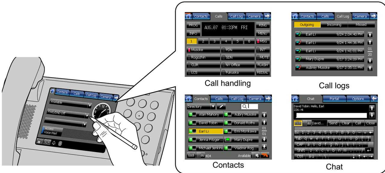
The large, color LCD touch screen provides a simple interface for operating the KX-NT400. You can assign commonly used phone numbers and functions to flexible keys for easy access. You can also check messages, missed calls, and more simply by pressing buttons on the screen. The touch screen also provides an intuitive interface for managing contacts and call logs.
