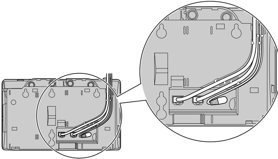
4. Drive 3 screws (included) into the wall as shown in the illustration below, and mount the KX-NT400 on the wall.
