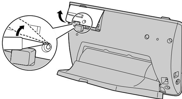
4. Install the KX-NT307 Bluetooth module to the Bluetooth module socket (see "Location of Controls (Page 18)").
