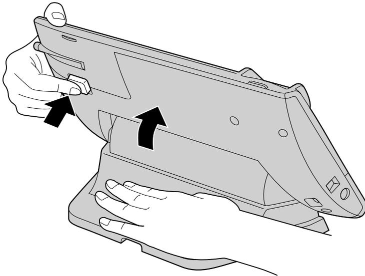
4. While holding down the button, tilt the board to the desired angle and then release the button.
