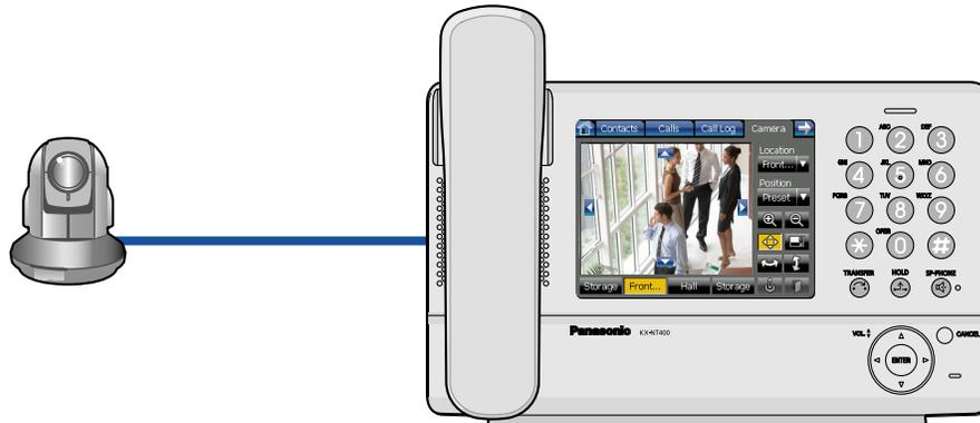
The KX-NT400 can display video feeds from Panasonic Network Cameras (e.g., KX-HCM/BB-HCM/BL-C series). You can register up to 20 cameras. If a registered camera is connected to a doorphone, whenever you make a call to or receive a call from that doorphone, the video feed is automatically displayed on the KX-NT400. In addition, you can register camera information with a contact, and view the camera's video feed when talking to the contact.
