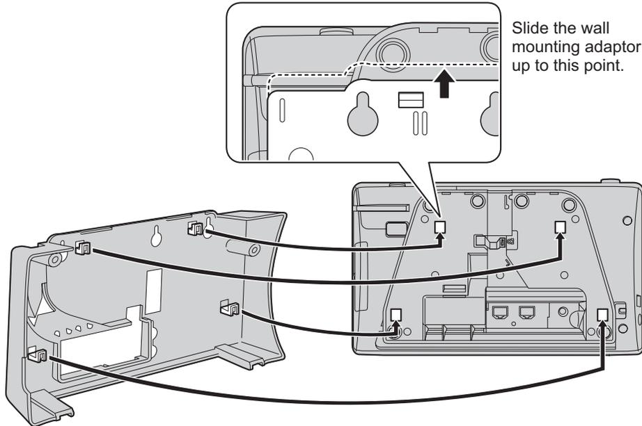
2. Fasten the wall mounting adaptor to the base with 2 screws (included).
