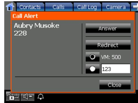
If you are viewing the **Camera** screen when an incoming call arrives, the **Call Alert** window appears along the bottom of the screen.
